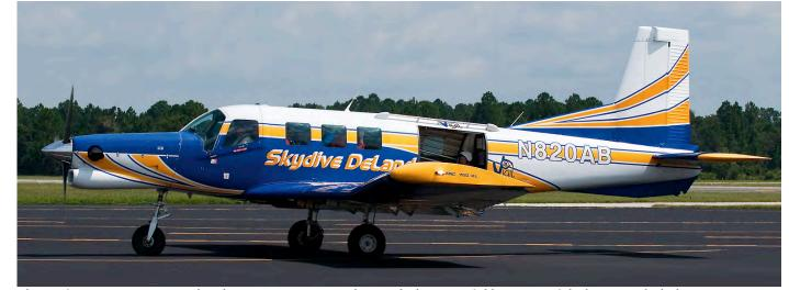
The Pacific Aerospace 750XL, marketed as P-750 XSTOL, is popular as a skydive aircraft, like N820AB of Skydive DeLand. The bent up outer wings are the distinctive characteristic of the single engine turboprop. (DeLand (FL), 28 July 2013, Joost de Wit)
