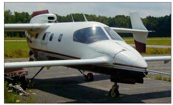
The OMAC Laser 300 is a high wing aircraft with a canard configuration. Its vertical stabilisers are at the wing tips. The aircraft has one turboprop engine in the rear fuselage, powering a pusher propeller. (*photo left column by Terry Shepherd*)
