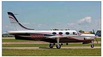
The Speedstar 850 is a heavily modified Piper Aerostar 602P with a single turboprop engine in the nose. N5530T was photographed at Oshkosh (WI) on 25 July 2010 by Joe Evens)
