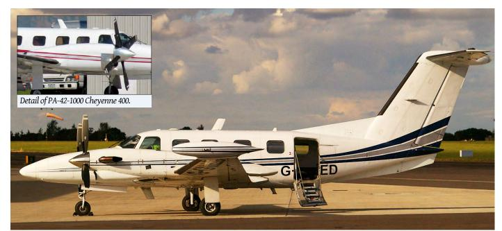
The Piper PA-42 Cheyenne III has a low wing with two turboprops and a T-tail like the Beech Super King Air. However they are easy to keep apart: the T-tail of the Cheyenne is much higher and the cabin windows are larger and rectangular. The detail shows the different engine cowlings of the Cheyenne 400, with TPE331 engines instead of PT6As. (G-GMED, Norwich, 14 September 2012, Bob Ward)
