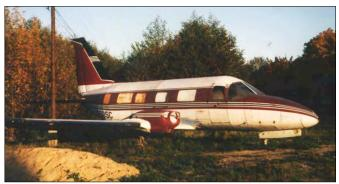
The Piper PA-35 looks like a "blown-up" Navajo, as it has a wider fuselage and a larger vertical tail. Just one such piston powered aircraft was built. (photo Hans Hoogers)
