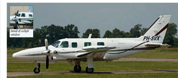
On this photo by Joost de Wit, the third square cabin window on the left side of the PA-31T2 Cheyenne IIXL is clearly visible, just after the cockpit side window. Also it can be seen that the cockpit front window has the same height as the side window. Compare this to the small photo of older Cheyenne models and you will see what we mean.
