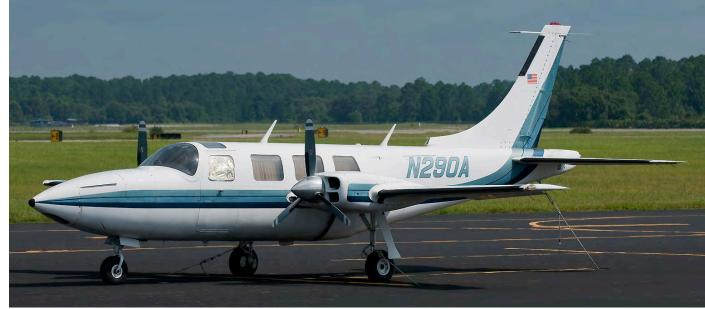
Of all the cabin class piston twins the Ted Smith Aerostar is the easiest to recognise, because of the wings going straight through the fuselage. N290A is an Aerostar 601P. (DeLand (FL), 28 July 2013, Joost de Wit)
