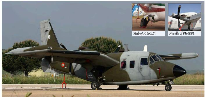
Being derived from the Piaggio P136 amphibian aircraft the P166 has a distinctive shape. There is no other high wing aircraft with pusher props. Many have ended up with the Italian military, like this P166DL3 MM25158 with Lycoming LTP101 turboprop engines. Note the large exhaust on top of the nacelles, compared to that of the P166DP1. (Pratica di Mare, 2 May 2012, Rob Hendriks)
