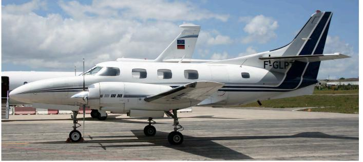
When you compare the Merlin IIA on the previous page to the Merlin III shown above, it seems like a completely different aircraft. In fact only the nose, gear, tail and engines nacelles are new. F-GLPT is an SA226T(B) Merlin IIIB, characterised by the small cabin window in the rear fuse-lage and the four-bladed props. (Lisbon, 12 May 2009, João Sa Pessoa)
