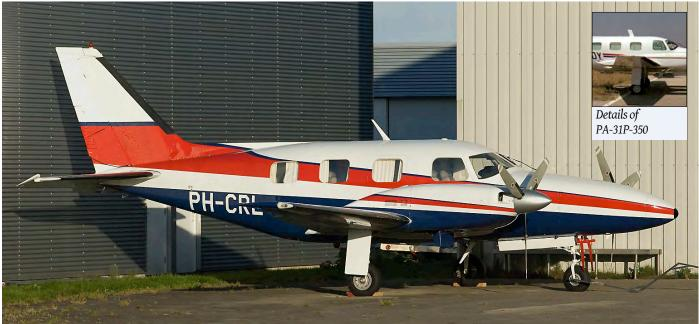
PH-CRL is a Pressurised Navajo, designated PA-31P. Compared to the original Navajo it has clearly smaller cockpit and cabin windows. Also the engine nacelles are shorter. The Piper PA-31P-350 Mojave (see inset) looks like the Pressurised Najavo, but has a larger cockpit side window and long nacelles.
