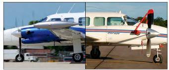
Engine nacelles of the PA-31T3 (left) and the Neiva NE821 (right). The latter is the same as for the Schafer Comanchero conversion.
