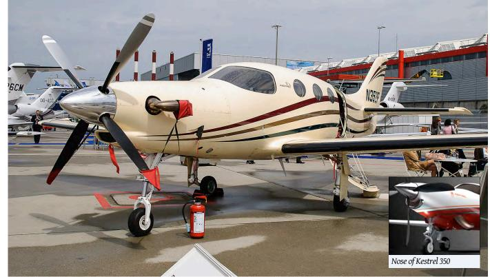
One Aviation, the result of the merger between Eclipse Aerospace and Kestrel Aircraft, aims to certify the Kestrel 350 single engine turboprop. The aircraft is based on the Farnborough F1 that is shown on the large photo. Compared to the F1 the 350 will have a TPE331 engine, which makes it easier to differentiate the Kestrel 350 from the similar Epic LT. (Geneva, 12 May 2009)
