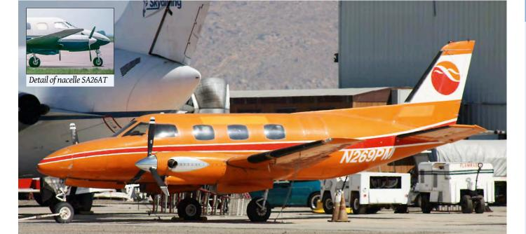
While the distinctive characteristics of the Swearingen Merlin/Metro series are visible, especially in the form of the cockpit and cabin windows, the heritage of the Beechcraft Queen Air is also apparent. Look for example at the landing gear and the tail. N269PM is an SA26T Merlin IIA, with PT6A engines, recognisable by the location and size of the exhausts. (Perris Valley (CA), 15 October 2011, Simon Titchmarsh)
