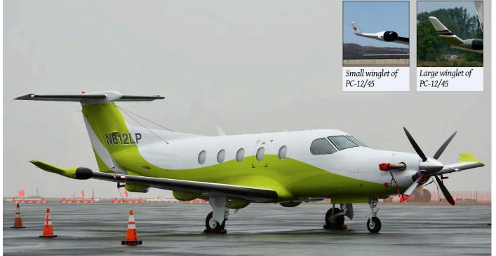
As the only single engine turboprop with a low wing and a T-tail the Pilatus PC-12 was easy to recognise, until the arrival of the similar looking Cessna Denali. N812LP shown is a PC-12/47E, the newest generation hence also marketed as the PC-12NG. The small photos show the two typical winglets of the PC-12/45. Which ones are fitted depends on the choice of the buyer. (Nashville (TN), 24 March 2013, Roy Gorris)
