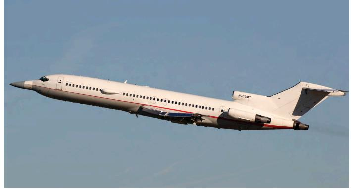
Raytheon Flight Test Operations is listed as operator for this 1981-built B727-200. As the humps and bumps indicate, the test purpose as Raytheon uses this classic for testing the F-35 radar. Flying out of LAX Voodoo1 graces the skies between all modern Boeing and Airbus airlines. (8 November 2017, Eric Vangeel)
