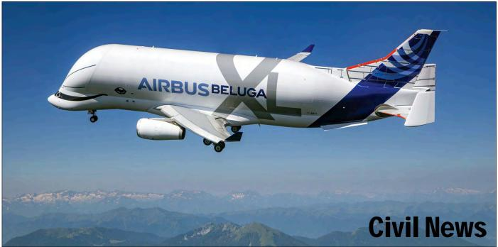
On Thursday 19 July 2018 the new Airbus BelugaXL made its first flight. The BelugaXL is based on the Airbus A330-200 and is officially designated as A330-700L. Airbus is planning to build four BelugaXLs, which will replace the current five BelugaSTs in their fleet. The test aircraft was registered as F-WBXL and sported special "White Whale" markings. (In flight, 19 July 2018, Airbus - S. Ramadier).
