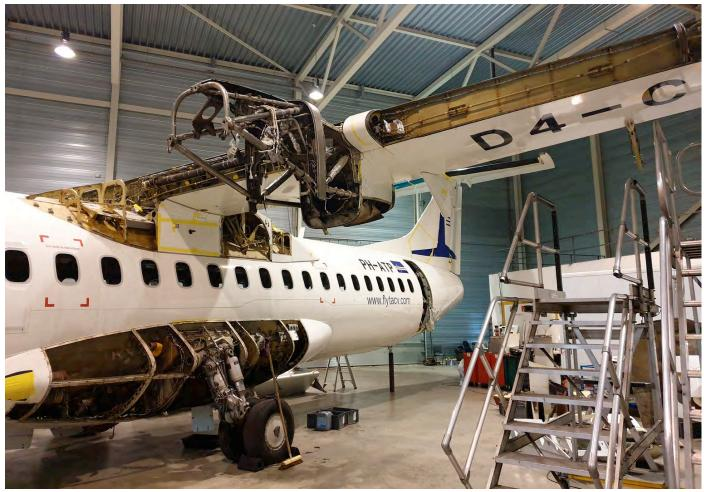
ATR72 PH-ATP arrived at Maastricht on 3 October 2017 registered as D4-CCC. After having been stored at the airport it was caught on camera while being dismantled. Usable parts have been salvaged. What remains has been transported to PS Aero in Baarlo. There the fuselage will be converted into an attraction. (Maastricht - Aachen, 26 January 2019, Danny Versteegen)
