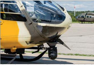
Close-up showing the FLIR installation, which is only fitted to the aggressor Lakotas, on UH-72A 09-72107. (25 August 2021)
