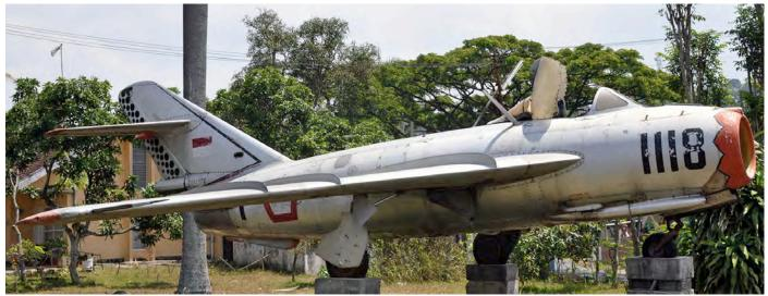
Note the drag-chute compartment below the rudder. These were added on some aircraft during their operational career. Maybe during rehabilitation in the late 60's. F1105, F1109 and F1118 (also see photo earlier, note that the red serial is now black) are photo proof. (Desa Polaman, 23 August 2009, Marco Pennings)
