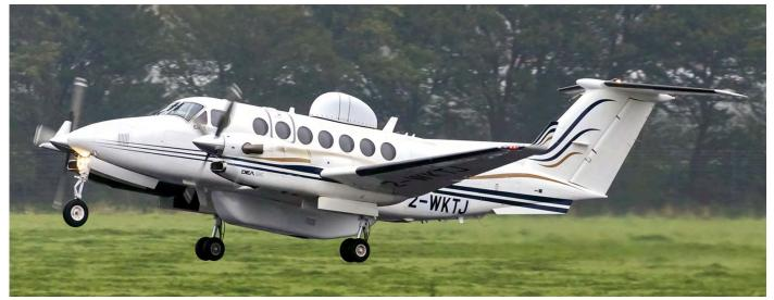
This Super King Air 350 2-WKTJ (with msn FL-470) was registered into the register of Guernsey in October this year and is operating for Diamond Executive Aviation. This aircraft has been used since as an airborne relay- and measurement aircraft, as can be seen by the extra dome on top and extra belly under the fuselage. (Rotterdam - The Haque, 1 November 2019, JvL.Holland)
