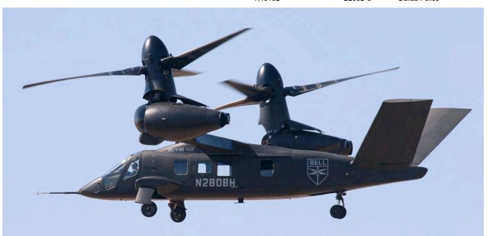
The Bell V-280 Valor is a tilt-rotor aircraft being developed for the US Army Future Vertical Lift Program. It is intended to replace various types within the US Army. (20 October 2019, Ft. Worth-Alliance (TX), Otger van der Kooij)
